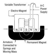
Figure 1. Eriez Magnetic Drive Circuit
