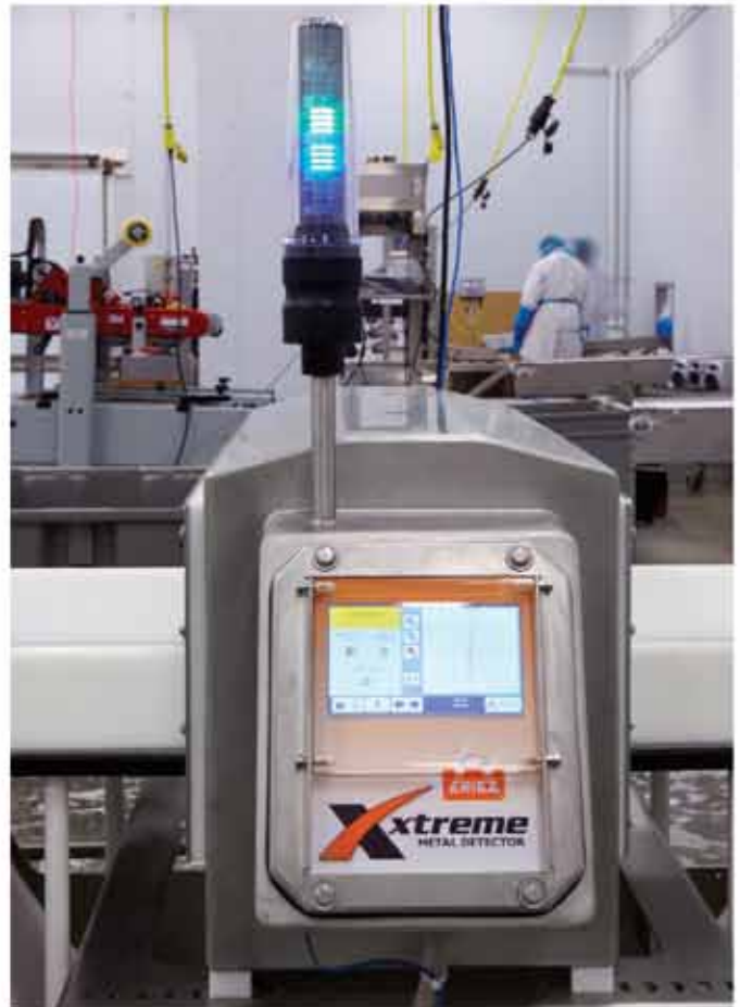
The new Xtreme® Metal Detector pushes the detection/productivity curve with the ability to detect 0.2mm spheres.
