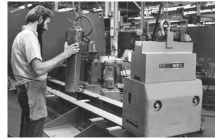
Eriez Bi-Polar Magnets, with a wide range of optional pole-plate configurations, are ideally suited for handling pipe, rounds, bundles, angles and shapes. They can be used in single- or multiple-magnet applications.
