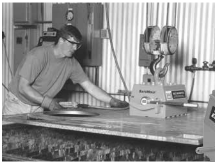
EPL Series SafeHold® Magnets are ideal for many machine-shop operations including the loading and unloading of this burn table.
